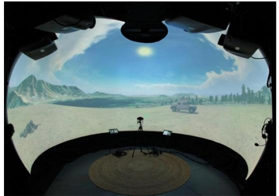
The core AJTS configuration consists of a domed visual display system with high resolution projectors, a powerful and intuitive Computer Generated Force (CGF) / Semi-Autonomous Force (SAF) application, a high fidelity Image Generator (IG) system capable of rendering scenes in multiple spectrums, a dynamic aural cueing system, and a full suite of emulated, stimulated, and virtual military equipment.
